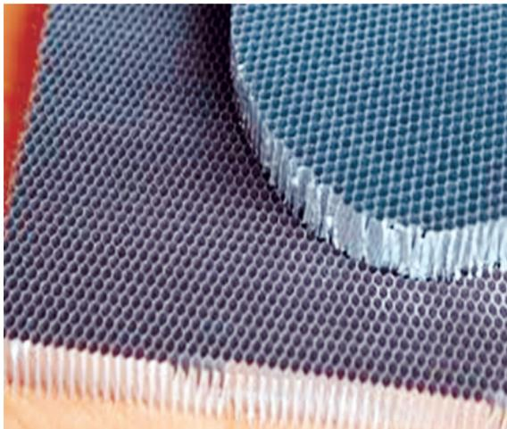
**Fig. 7.** Honeycomb structure.
