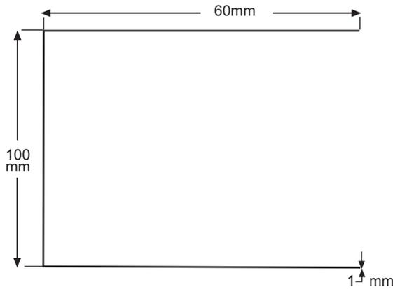
**Fig. 1.** Cross section showing the dimensions of designed cold-form C section beam.
