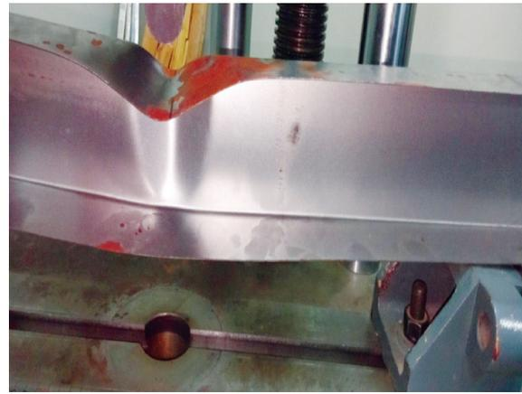
**Fig. 10.** Deflected shape of specimen with the application of load.
