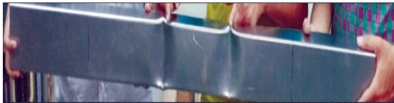
**Fig. 15.** Deflected beam under two-point load test.
