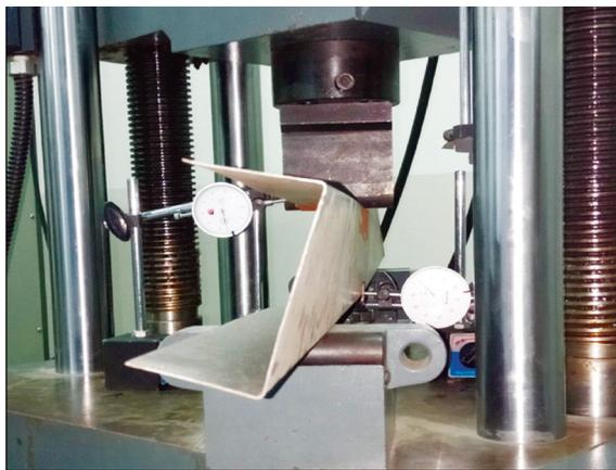
**Fig. 9.** Deflection of beam under applied load.
