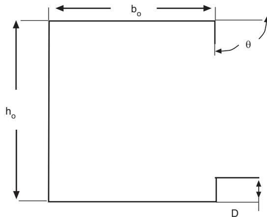
**Fig. 4.** Symbols used in prequalification of cold-form beam.
