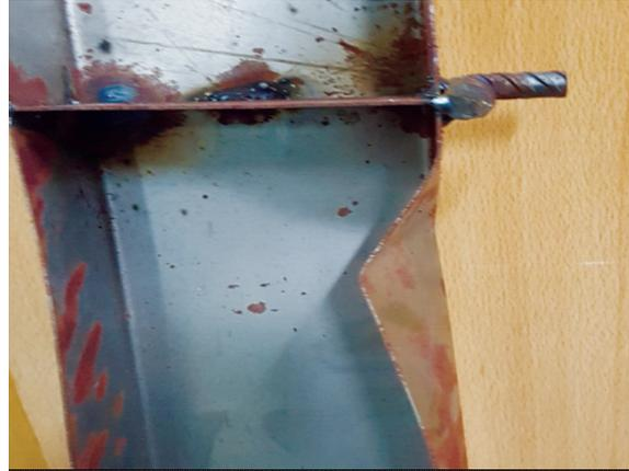
**Fig. 12.** One point load test on flange of C section with applied on shear center of beam using heavy stiffeners.
