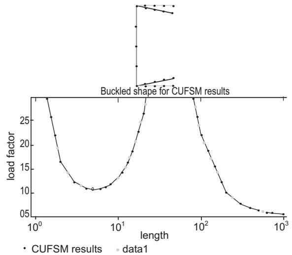
**Fig. 6.** Analysis results of beam in CUFSM 5.
