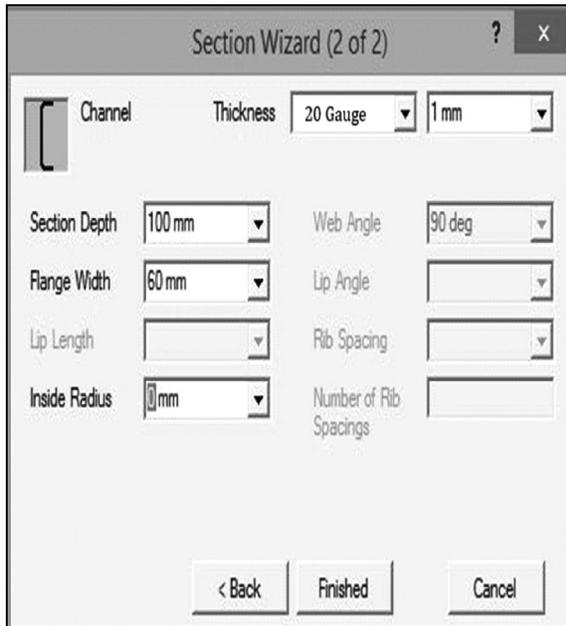
**Fig. 2.** Cold-form beam data input dialog box in CFS10.
