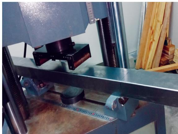
**Fig. 14.** Placement of specimen in UTM in two-point load on web settings.
