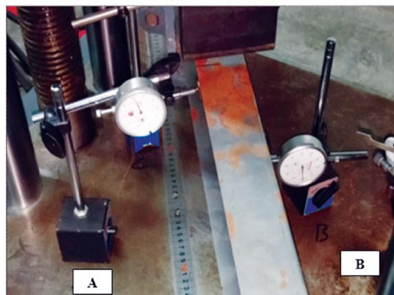
**Fig. 7.** Installation of dial gauges 'A' and 'B' on the designed beam.
