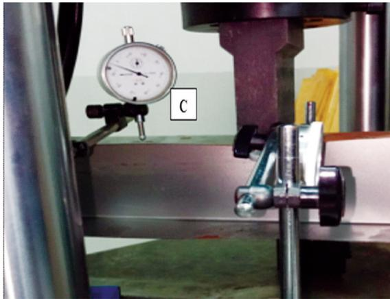
**Fig. 8.** Assembly of dial gauge 'C' on the designed beam.
