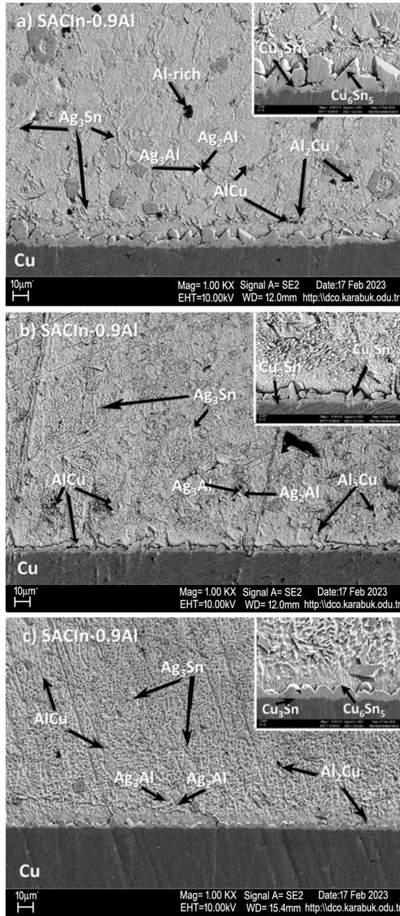
**Fig. 7.** SEM analysis of SAC205-1In-0.9Al at different temperatures: (a) 275 °C, (b) 300 °C, (c) 325 °C.
