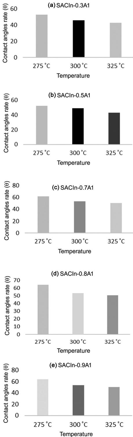
**Chart 1.** shows the contact angle rates of lead-free solder alloys produced at 275 °C, 300 °C, and 325 °C. 15<sup>th</sup>, 30<sup>th</sup>, 60<sup>th</sup>, 90<sup>th</sup>, 120<sup>th</sup>, 150<sup>th</sup>, 300<sup>th</sup> and 600<sup>th</sup> sec.
