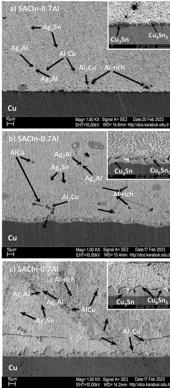
**Fig. 5.** SEM analysis of SAC205-1In-0.7Al at different temperatures: (a) 275 °C, (b) 300 °C, (c) 325 °C..
