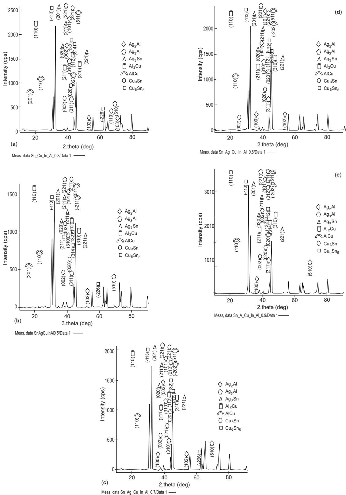
**Fig. 2.** XRD analysis of lead-free solder alloys SACIn-xAl shows the formation of intermetallic compounds: (a) SACIn-0.3Al, (b) SACIn-0.5Al, (c) SACIn-0.7Al, (d) SACIn-0.8Al, (e) SACIn-0.9Al.
