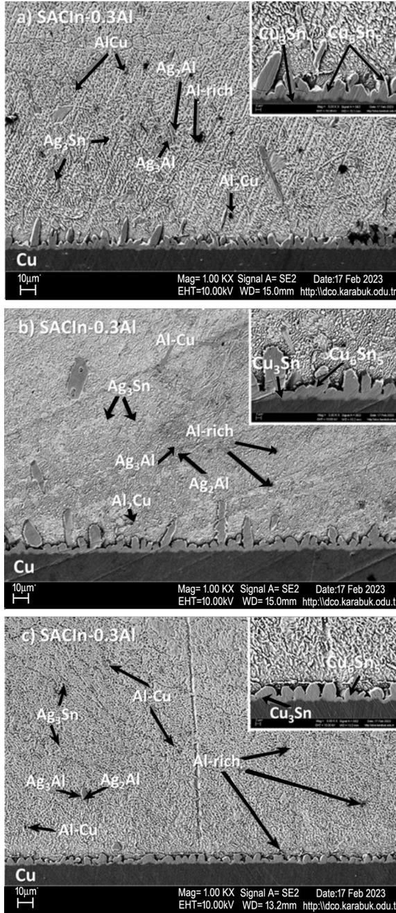
**Fig. 3.** SEM analysis of SAC205-1In-0.3Al at different temperatures: (a) 275 °C, (b) 300 °C, (c) 325 °C.
