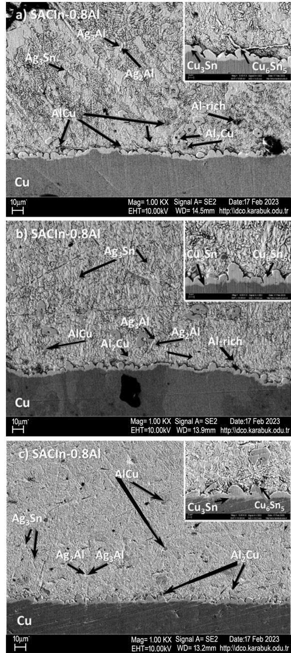
**Fig. 6.** SEM analysis of SAC205-1In-0.8Al at different temperatures: (a) 275 °C, (b) 300 °C, (c) 325 °C.
