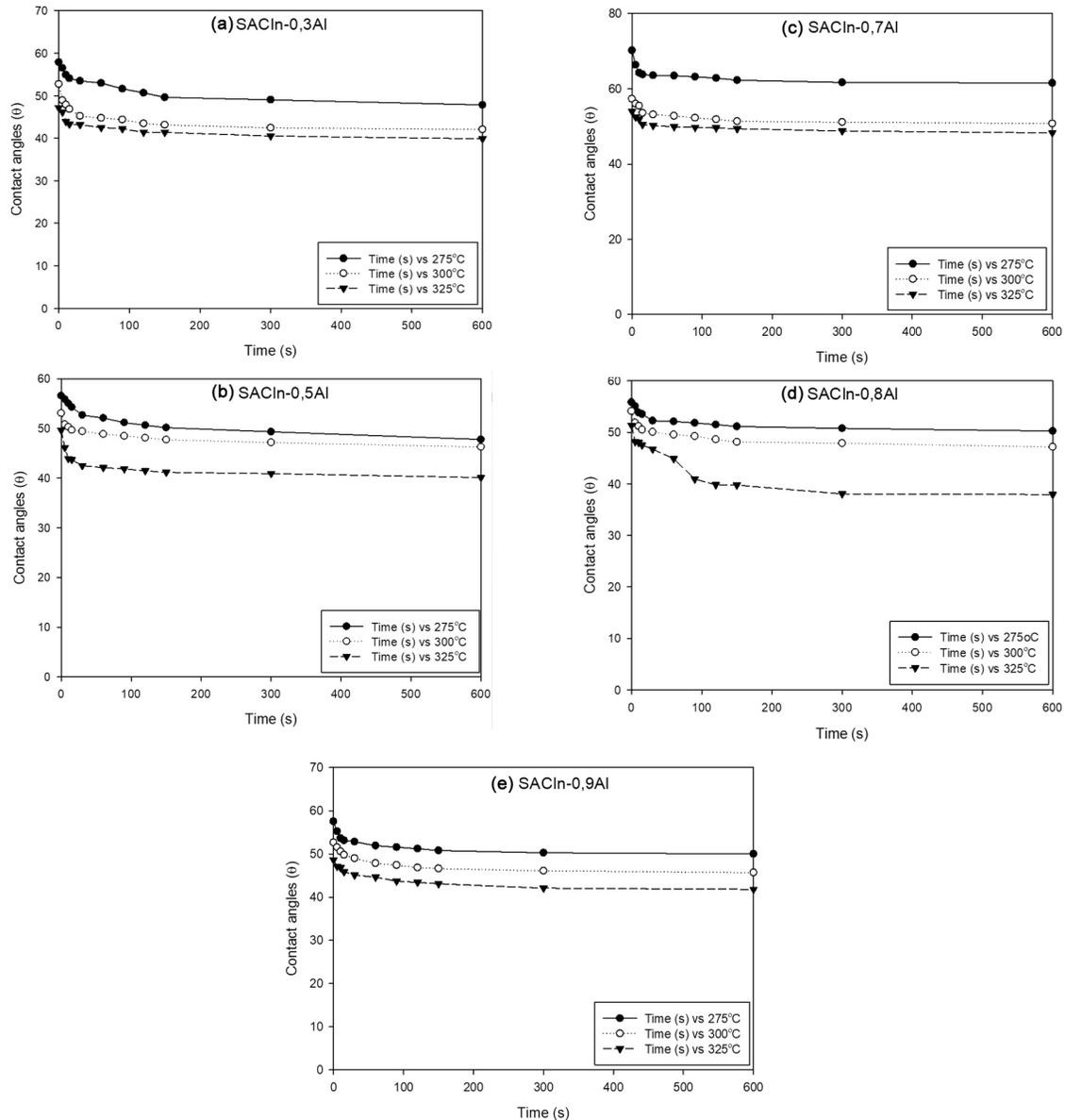
**Fig. 1.(a,b,c,d,e)** shows the average of contact angles (both left and right) from three positive experiments at different time intervals, including 5<sup>th</sup>, 10<sup>th</sup>, 15<sup>th</sup>, 30<sup>th</sup>, 60<sup>th</sup>, 90<sup>th</sup>, 120<sup>th</sup>, 150<sup>th</sup>, 300<sup>th</sup> and 600<sup>th</sup> sec.
