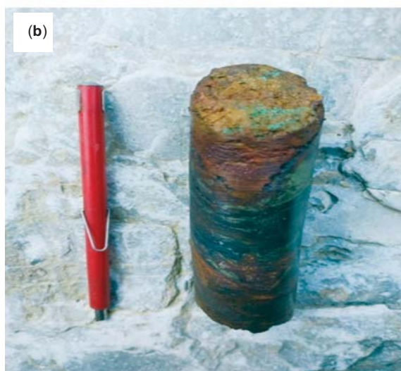
Fig. 11. Illustrations showing (a) Drilling operation within the study area using shaw portable drill rig (b) Collected oxidized core sample showing primary and secondary sulfide mineralization.
