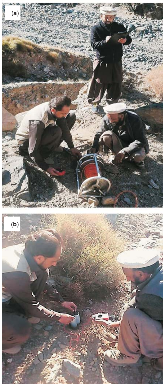
Fig. 4. Field photographs showing (a) SP data measurement using a digital multimeter during the field work (b) Measurement of base to roving pot drift voltage at the base station.
