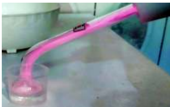
Fig. 4. Mushroom probe filled by Neon gas and plasma produced after applying high voltage to the probe.
