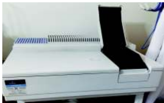
Fig. 6. PerkinElmer Lambda 25, used to detect the spectrum of species in active liquid.
