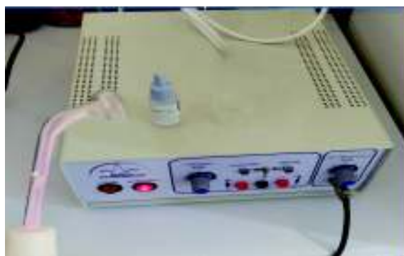
Fig. 2. High frequency, high voltage power supply in which was made by "Dorsa hydroderm company and mushroom electrode.
